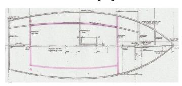
Full width bulkhead front of cockpit. Full or partial width rear cockpit bulkhead.
