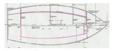
Full width bulkhead forward of mast Full or partial width rear cockpit bulkhead.
