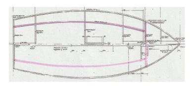
Full width bulkhead forward of mast Side tanks from bulkhead to transom.
